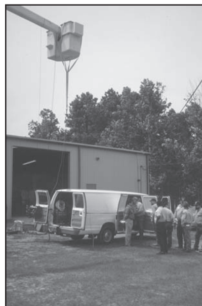
Figure 19. Stress load testing of bucket trucks demonstrated at the 2000 Contact Representative's Meeting.
